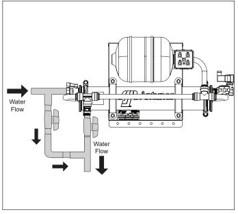
Figure 6. Install Bypass
