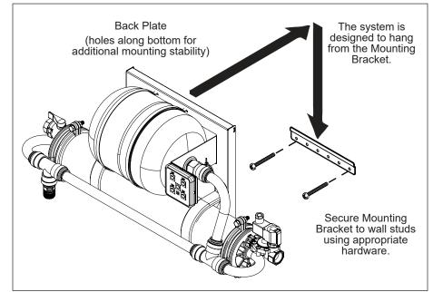
Figure 2. Mounting the System
