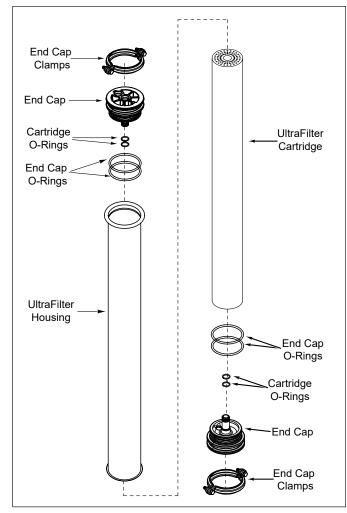
Figure 7. Replacing the Ultra Filter Cartridge
