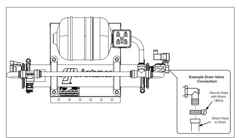
Figure 3. Drain Valve Connection
