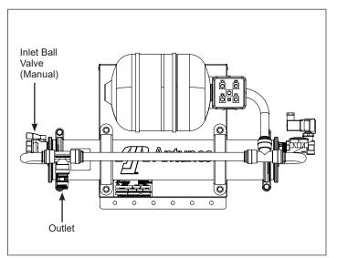
Figure 5. Inlet and Outlet Connections
