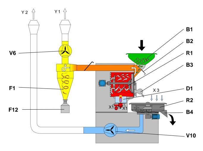
Illustration 2: Process scheme (variant 2: roasting/cooling exhaust air separated)
